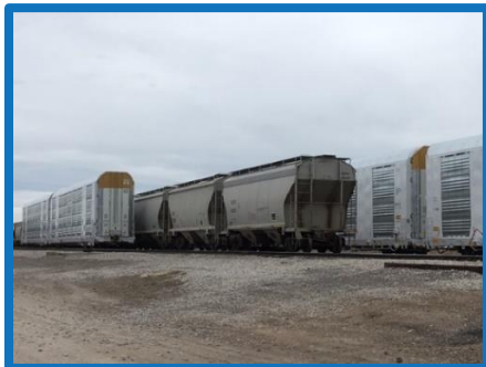
Auto Carrier Rack Cars with C4 Covered Hoppers (middle) at San Angelo TXPF Classification Yard, January 2020
