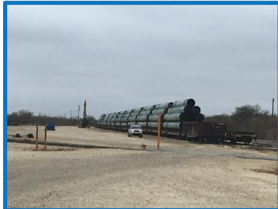
TTX 89' Flat Cars in Barnhart, Texas transiting pipe west
